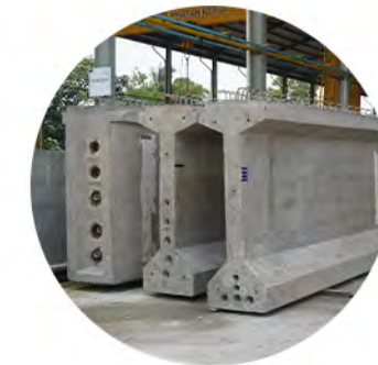
Type PC-I Girder H:2.1 L:40.8 M 20.957 Ton/Year
